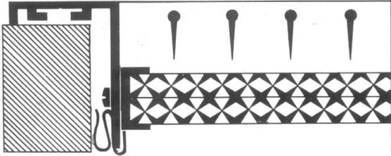
2) Visible screw fixing
